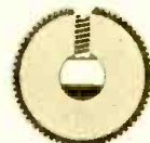
How shaft is positioned for set-screw knob.
