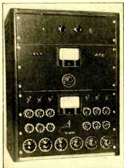
Fig. 1. The completed Semi-Professional Recording-Playback Amplifier. Identification of the equipment on the 3 panels (reading from left to right): Top Panel: "B" supply pilot and switch; "A" supply switch, and pilot. Middle Panel: off-1p of triodes Nos. 1 and 2; power level VU meter; off-plus 30 VU and 40 VU; (center knob) amplifier gain control. Bottom Panel: consider these controls in vertical rows, the first 5 of which are channel controls, bottom to top, as follows: channel volume control, L.F. control, H.F. control, dialogue filter switch. Row 6: master volume control, monitor volume control, expander control, monitor-compressor switch. The meter is a vacuum-tube VU type; underneath is the VU range selector switch; the 3 buttons underneath read: Monitor, Recording and Playback.
